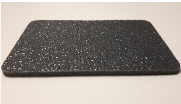
Fig.3 Photo of a typical polyurea sample with non-slip surface [2]
